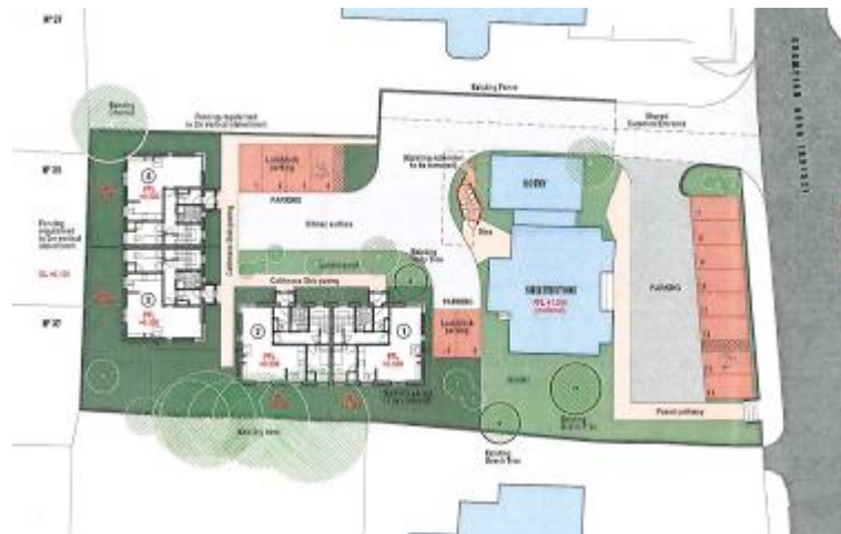
Fig 5 : Proposed site layout plan
